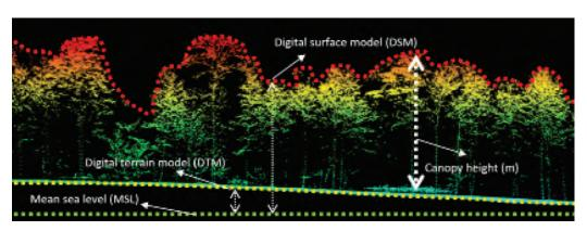
Figure 8.2: Example of cross-section through LiDAR point cloud
