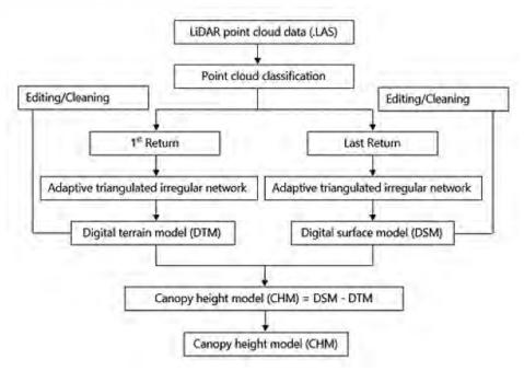
Figure 8.1: LiDAR point cloud data processing workflow for CHM extraction
