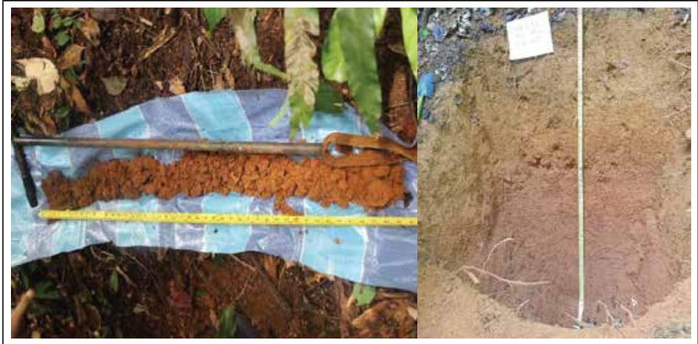
Figure 5: Soil profiles obtained from selected points within HoB's Pueh Expedition site using Edelman Auger (left) and pit digging (right)
